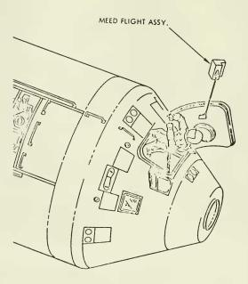
Figure 1. The MEED deployment in space from the Apollo 16 Command Module.
